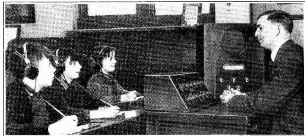
Multiple channel deaf aid system in use at the Hugh Middleton School for deaf and dumb children. The class is for partially deaf subjects and the teacher is able to control the volume and response independently for each pupil.
