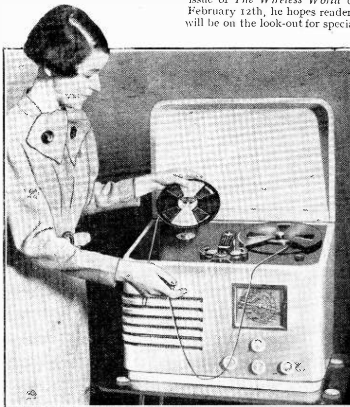
THE DUO-TRAC SOUND PROJECTOR, which is being shown and demonstrated at the British Industries Fair at Olympia, has the sound recorded on a film which gives 30 minutes' playing time with a spool of standard size. The apparatus shown above is a table model and embodies an all-wave radio chassis.
