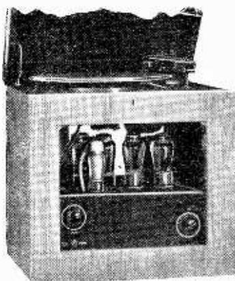
Amplifier and gramophone unit of portable equipment made by Francis, Day and Hunter.
