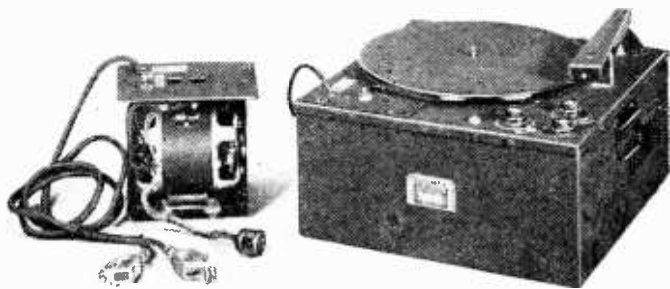
Rothermel mobile PA amplifier and alternative power unit for battery operation
